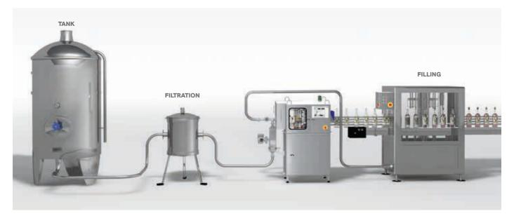
The Velcorin<sup>®</sup> dosing unit is installed in new or existing filling lines, and can be used for tank-to-tank treatment or upstream of the container filling system. Only minor modifications to the filling line are required for this purpose.
