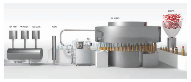
The Velcorin® dosing pump is installed in new or existing filling lines. Only minor modifications to the filling line are required for this purpose.
